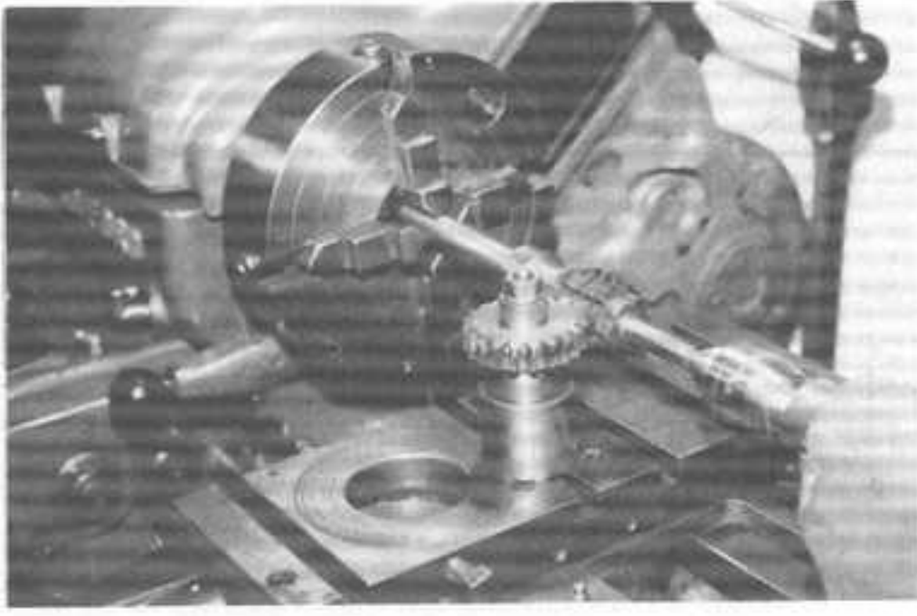
Fig. 79 "Free" Hobbing a worm in the lathe. The blank has first been 'gashed' to remove most of the material and to correctly space the teeth.
